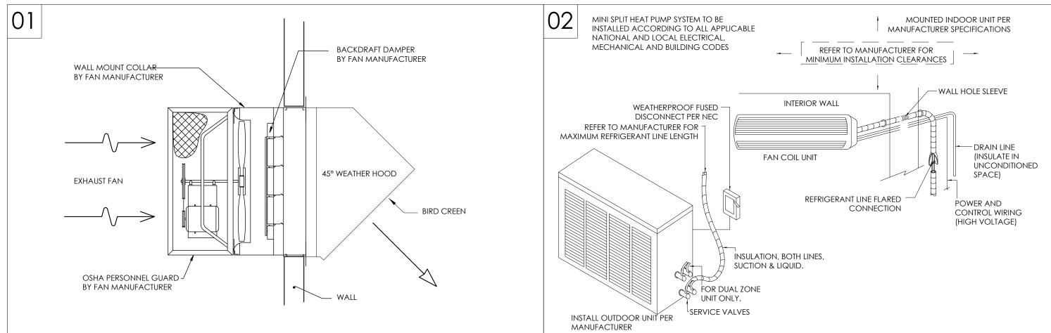
WALL PROPELLER FAN DETAIL
