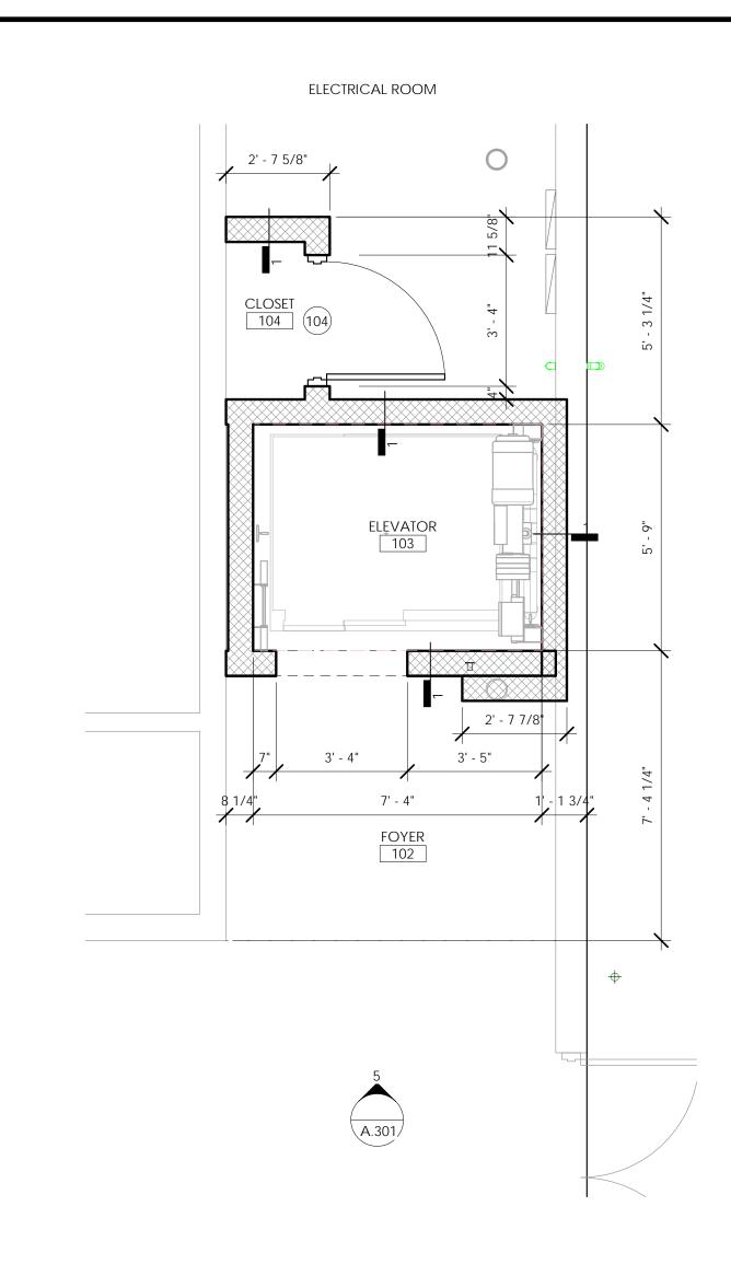
1 ENLARGED FIRST FLOOR PLAN - ELEVATOR ALT #1 A.301 SCALE: 3/8" = 1'-0" REF: A.101
