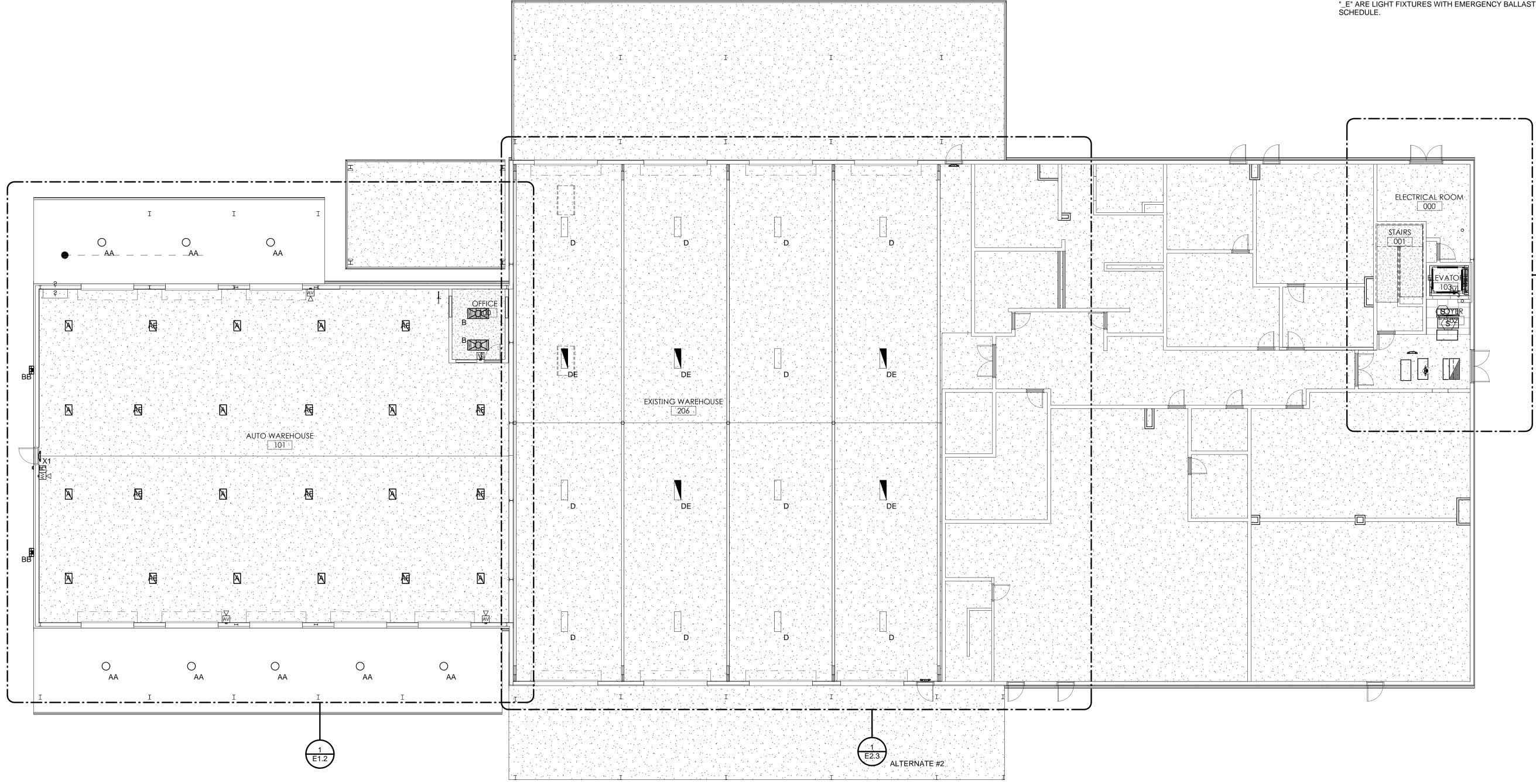
1 ELECTRICAL LIGHTING PLAN - OVERALL FIRST FLOOR E1.1 SCALE: 3/32" = 1'-0"REF:
